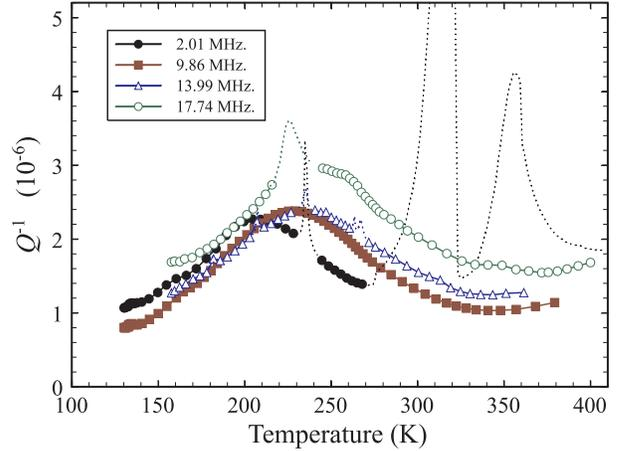
Figure 2:  $Q^{-1}$  versus temperature in specimen LGT7. Anomalous peaks are plotted with dotted lines.
