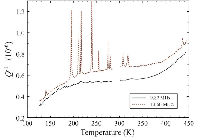
Figure 3:  $Q^{-1}$  versus temperature in specimen LGT17
