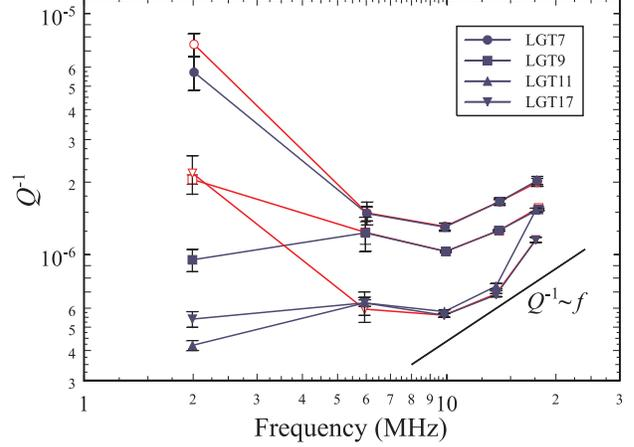
Figure 1:  $Q^{-1}$  of specimens with and without an O-ring resting on the upper surface. Filled symbols in the legend are for the measurements without the O-ring. Open symbols with the same shapes are used for measurements with the O-ring.
