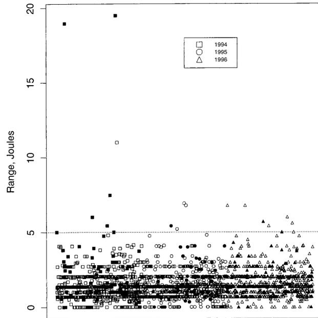
**Figure 5.** The range of the five specimens for the low-energy verification test. The horizontal axis is the sequence of the test. The order within each year is not relevant. The dotted line indicates the 5 J proposed rule. The solid markers designate the machines that fail the  $\pm 1.4$  J criteria.
