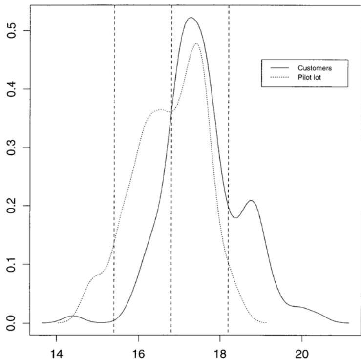
**Figure 2.** The density plots of the energy absorbed for the pilot lot data (from 75 individual specimens) associated with Lot 54. The three vertical dashed lines correspond to the reference energy (16.8 J) and the acceptance region ( $16.8 \pm 1.4$  J).
