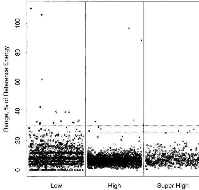
**Figure 7.** The normalized range of the five specimens for all the three energy verification tests. The solid markers designate the machines that fail the  $\pm 1.4$  J or  $\pm 5\%$  criteria. The dotted lines, at 25% and 30 %, are possible values of  $r$  to use in the range value.
