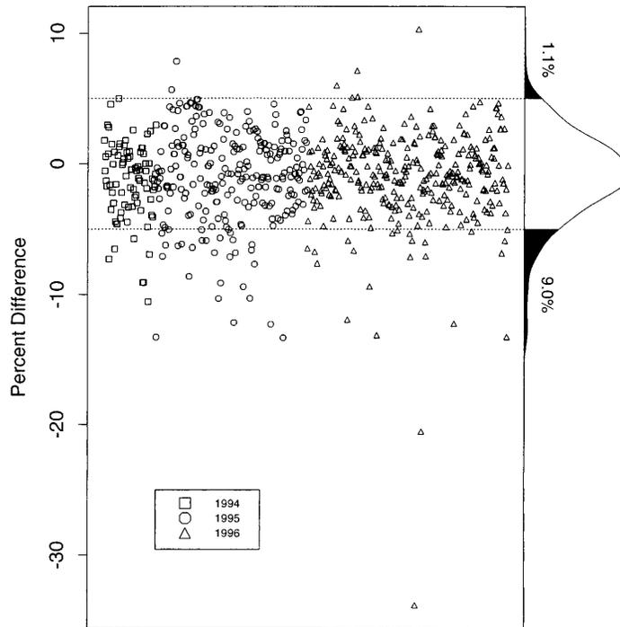
**Figure 4.** The relative difference between the customer's average for super-high-energy verification tests and the reference value. The horizontal axis is the sequence of the test. The order within each year is not relevant. The dotted lines indicate the 5% pass/fail criteria. The density estimate for the relative difference is plotted in the right margin.
