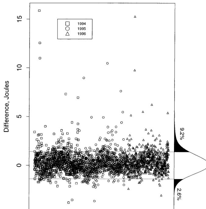
**Figure 1.** The difference, in J, between the customer's average for low energy verification tests and the reference value. The horizontal axis is the sequence of the test. The order within each year is not relevant. The dotted lines indicate the 1.4 J pass/fail criteria. The density estimate for the differences is plotted in the right margin.
