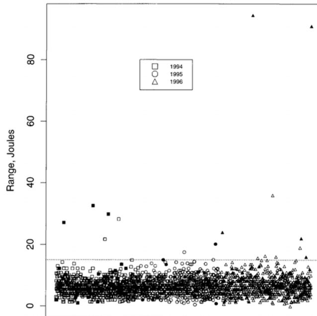
**Figure 6.** The range of the five specimens for the high-energy verification test. The horizontal axis is the sequence of the test. The order within each year is not relevant. The dotted line indicates the 15 J proposed rule. The solid markers designate the machines that fail the  $\pm 5\%$  criteria.
