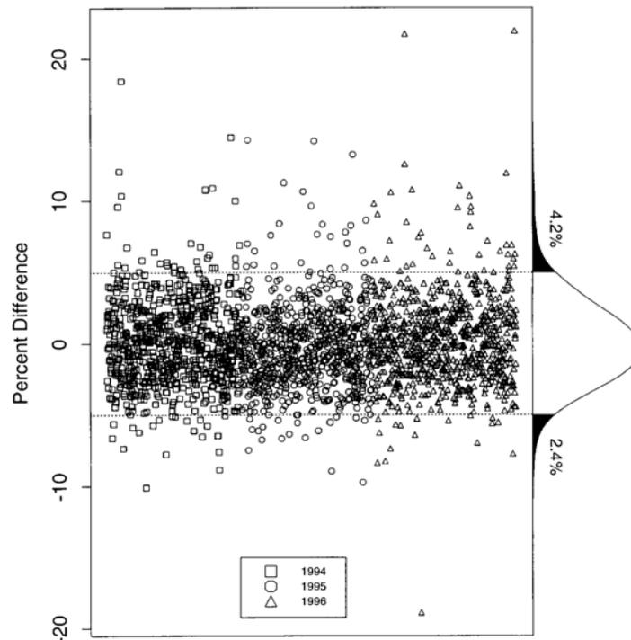
**Figure 3.** The relative difference between the customer's average for high-energy verification tests and the reference value. The horizontal axis is the sequence of the test. The order within each year is not relevant. The dotted lines indicate the 5% pass/fail criteria. The density estimate for the relative differences is plotted in the right margin.
