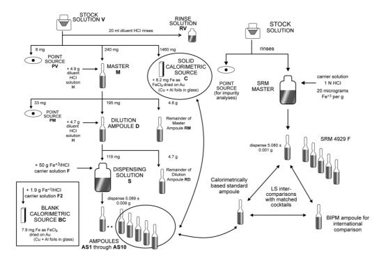
*Fig. 1.* Scheme for the primary calorimetric standardization of <sup>55</sup>Fe as used for SRM 4927 and for the BIPM international measurement comparison, showing the gravimetric links between the solid calorimetric source and the various <sup>55</sup>Fe solution ampoules
