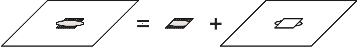
Figure 1. Schematic of the problem considered and the approximation that is made in this paper. The square grating target is over-illuminated by a Gaussian beam (ellipse). The field scattered by the system is treated as the sum of the diffraction by the square target and that of the region outside the target.
