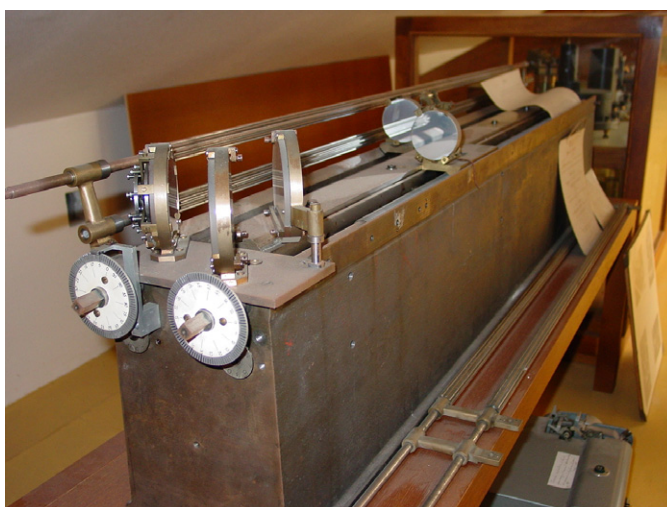
Figure 3. Photograph of a Michelson interferometer at BIPM used by Michelson for dimensional metrology with light. It seems that this same instrument was used in about 1970 by Barger and Giacomo to make wavelength comparisons between the ^{86}\text{Kr} lamp that served to define the metre and a methane stabilized 3.39\ \mu\text{m} HeNe laser. (2003 photo with permission from Tai Hyun Yoon, KRISS, Korea).
