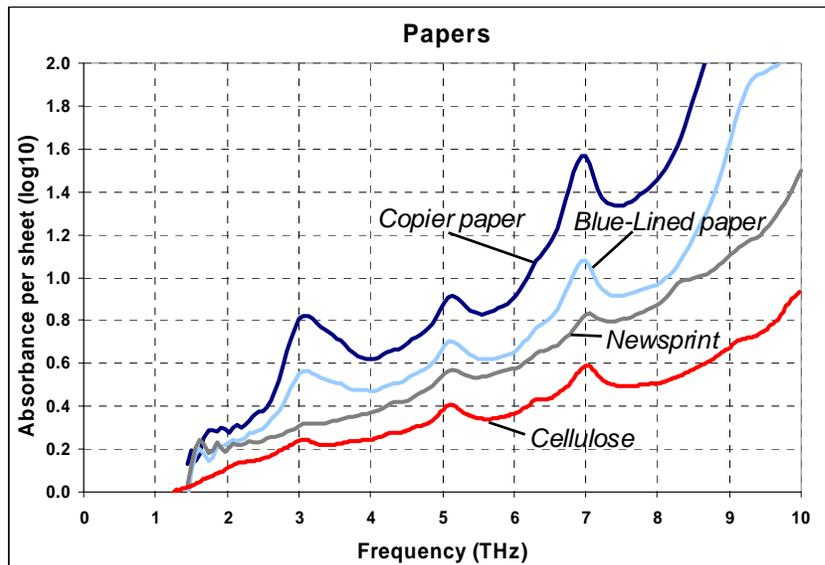
Figure 3 – Absorption spectra of different types of paper and cellulose
