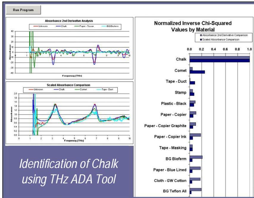
Figure 4 - Screenshot of the ADA Tool output demonstrating the ability to accurately identify materials housed in sealed containers by only considering the THz transmission spectrum of the container.
