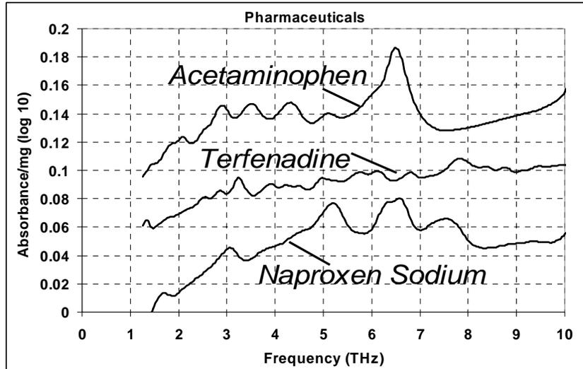
Figure 2 – Absorbance spectra for three pharmaceuticals measured with the FT-IR
