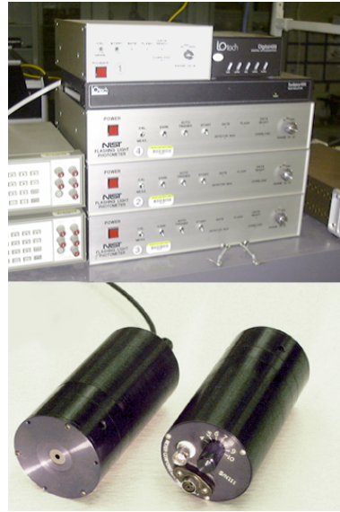
Figure 4. NIST flashing-light standard photometers (below) and the current integrator units (above).
