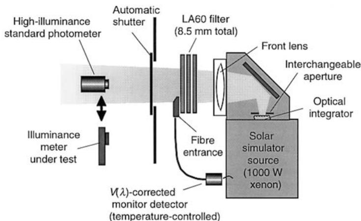
**Figure 2.** Configuration of the high-illuminance calibration facility (top view).
