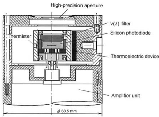
**Figure 3.** Design of the NIST temperature-controlled photometer used as high-illuminance reference standard.
