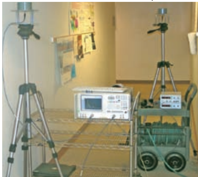
FIGURE 3. UWB Channel Sounder Developed at NIST
