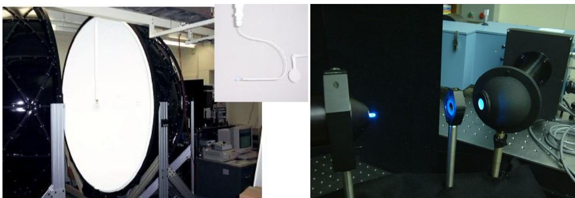
Fig. 7. NIST 2.5 m integrating sphere and the LED mount.
