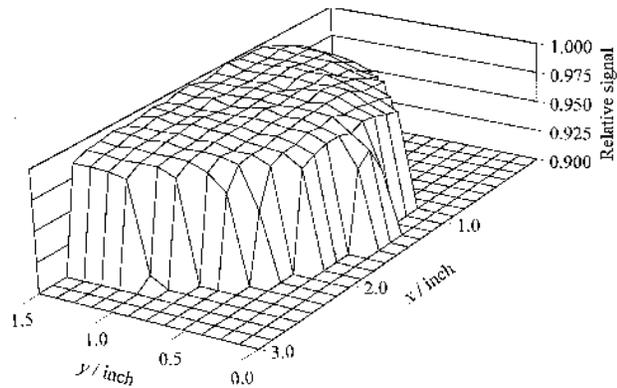
**Figure 5.** Three-dimensional representation of the radiance-meter detection of the output of the 200 mm (8") integrating sphere with a 64 mm (2.5") exit port. The data were obtained by computer-controlled manipulation of translation stages. The signal has been normalized and the bottom 90 % has been masked to accentuate nonuniformities. (The  $x$  and  $y$  axes are scanned in inches.)
