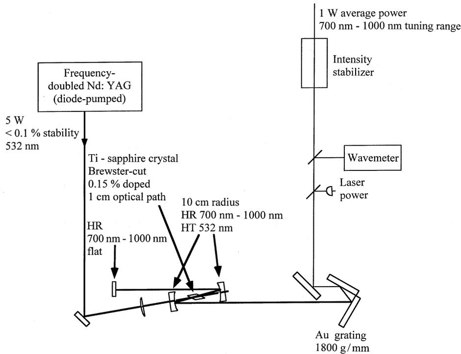
**Figure 2.** Ti-sapphire laser in its cw mode of operation. The laser is tuned by rotating the grating around an axis normal to the drawing. For the mode-locked version, the grating is replaced with an output coupler and the high-reflector end is replaced with twin fused-silica Brewster prisms for dispersion compensation. HR, high reflectivity; HT, high transmissivity.
