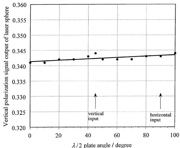
**Figure 6.** Polarized output of a 38 mm (1.5") laser sphere with 13 mm (0.5") output port obtained by varying the direction of the linearly polarized input beam with a  $\lambda/2$  plate. The drift shown by the linear least-squares fit is caused by the drift of the (unstabilized) He-Ne laser.
