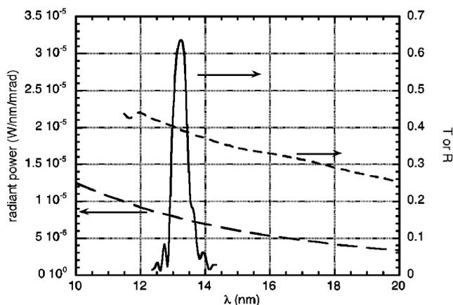
FIG. 2. Reflectance of multilayer mirror (solid line), transmittance of Be filter (short-dashed line), and calculated radiant power of SURF III (long dashes), which are used to calculate the incident spectrum and total throughput of the exposure beamline.
