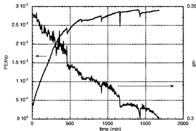
FIG. 4. Reflectance (squares) and normalized photoemission (circles) from a Mo/Si multilayer test sample.
