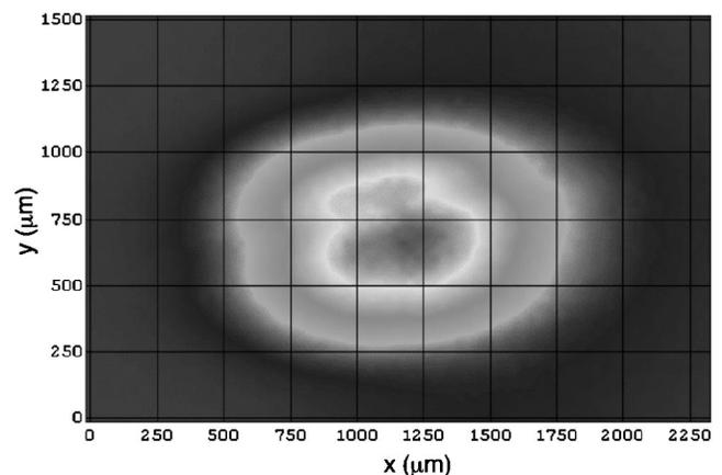
FIG. 3. Measured beam size at the sample plane, obtained using a Nd:YAG scintillator crystal with a 0.5 mm period reticle.
