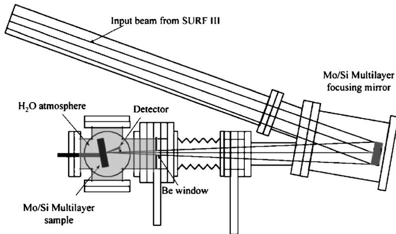
FIG. 1. Layout of multilayer exposure beamline.
