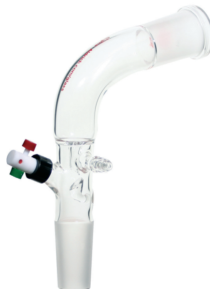
Figure 1: Distillate sampling adapter.
