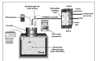
**Figure 1.** A schematic diagram of the cryoadsorber headspace sampling approach, configured for precise control and measurement of temperature and flow rate.
