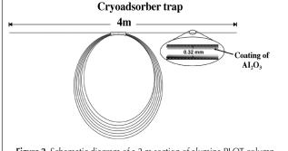
**Figure 2.** Schematic diagram of a 2 m section of alumina PLOT column used for the cryoadsorber.
