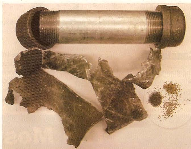
Figure 1 Pipe commonly used in IEDs and "exploded view" fragments of a pipe bomb generated by the FBI laboratory using smokeless powder.
