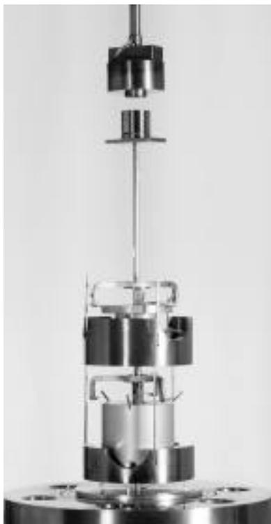
Figure 1. Sinkers and magnetic suspension coupling.
