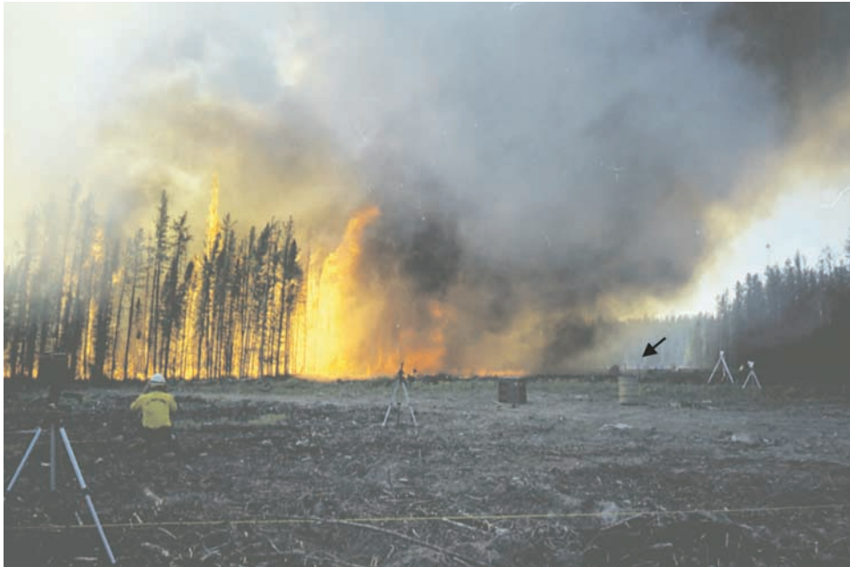
Figure 2. View of the 4 July burn as the flame front reaches the end of the plot and sooty smoke extends through the fireguard. Sampling equipment, located on the right side of the fireguard (arrow), is positioned to collect particles from the black plume near ground level shown in the photograph.
