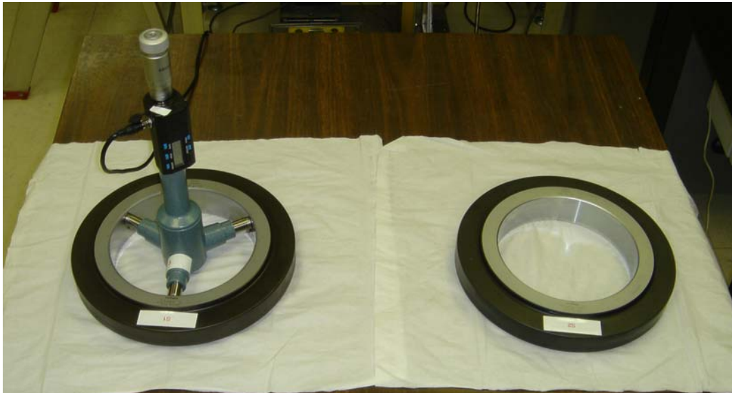
Fig. 1 The 3-point micrometer and two setting rings used for diameter measurements of the piston prover cylinder.
