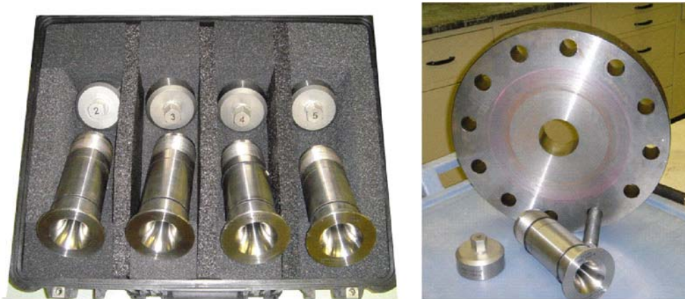
Fig. 1 The four critical venturis (“nozzles”) used as the transfer standard during the comparison.
