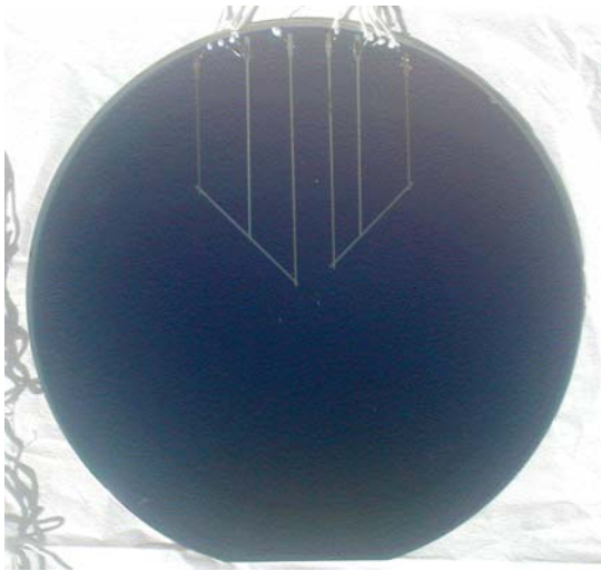
Figure 1. A photograph of a Pt/Rh thin-film thermocouple wafer used in the calibration.
