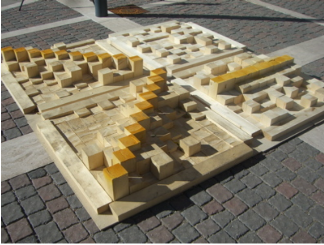
Figure 4: An arrangement of half-cubic (orange) stepfield pallets.
