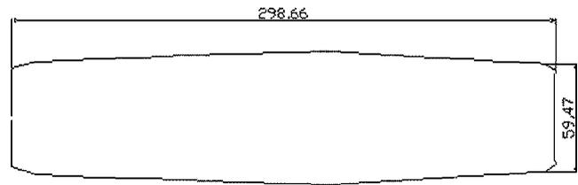
**Fig. 4** Beam footprint on the mandrel under test (units: mm).
