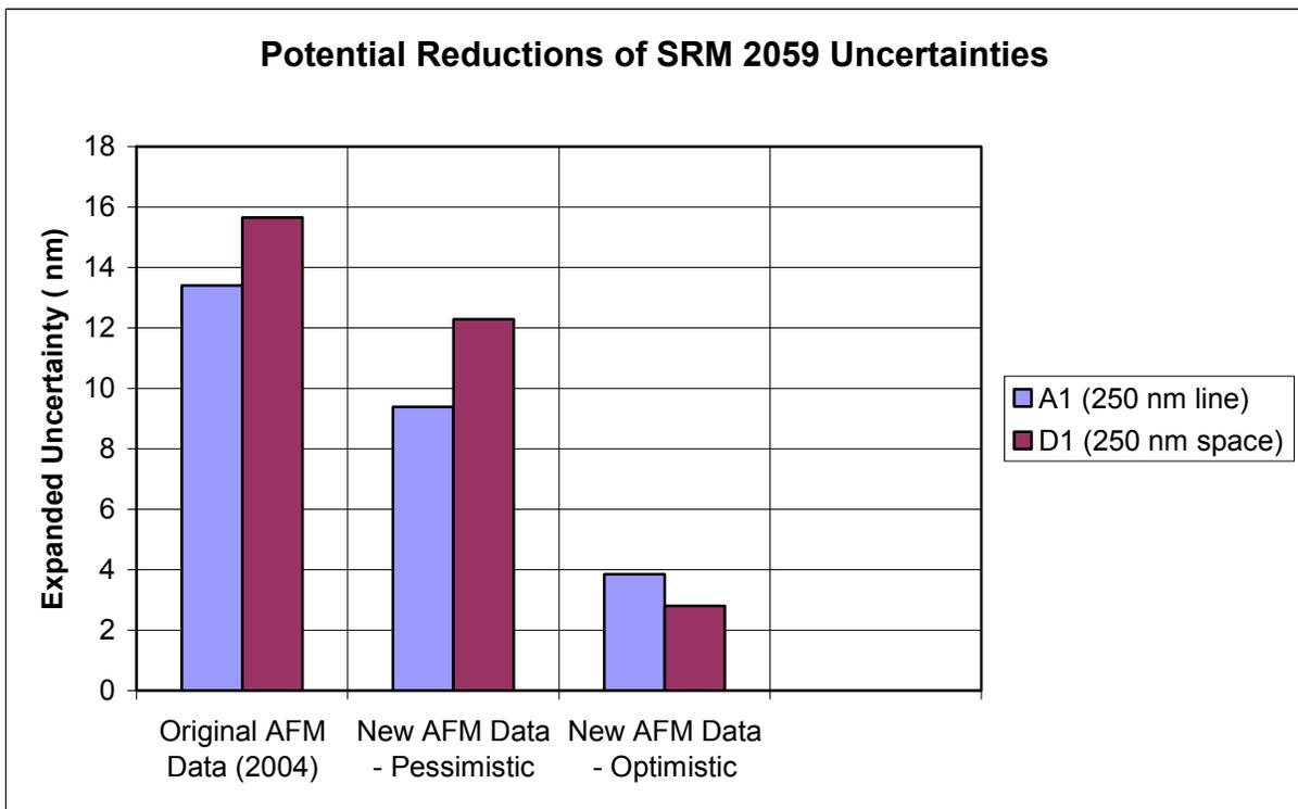
**Figure 6.** Original SRM 2059 uncertainties compared with optimistic and pessimistic estimates of final uncertainties based on the new AFM reference data.
