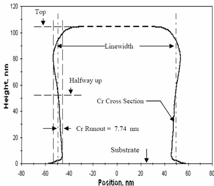
**Figure 2.** Composite CD-AFM cross-section of features on SRM2059. The irregular shape of some chrome-on-glass photomask features presents a greater challenge to CD-AFM metrology than typical poly-crystalline silicon structures. In particular, higher-order (e.g. shape) tip effects are a non-negligible source of uncertainty.
