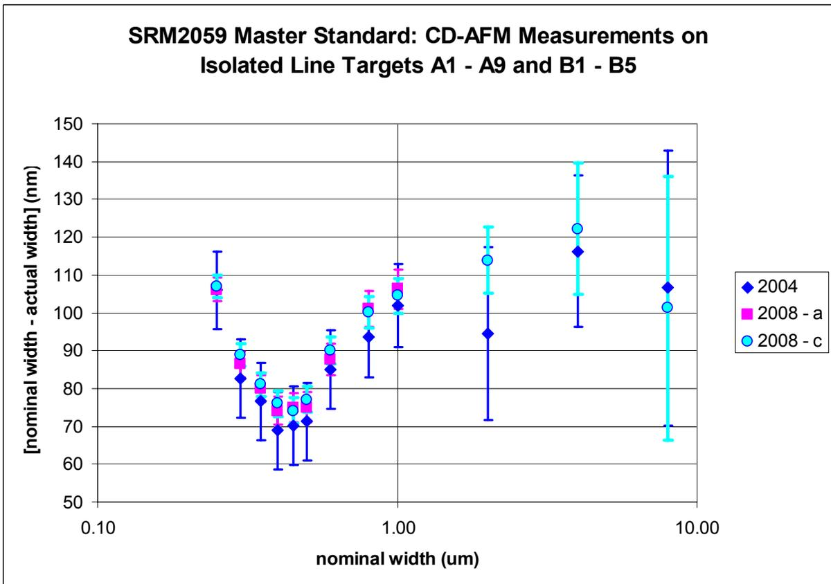
**Figure 4.** New and original CD-AFM reference measurement on the isolated line targets of SRM 2059 – ranging from 0.25 μm width (A1 feature) up to 8 μm (B5 feature). The error bars represent expanded ( $k = 2$ ) uncertainties, which have been reduced by approximately x4 for the smallest features.
