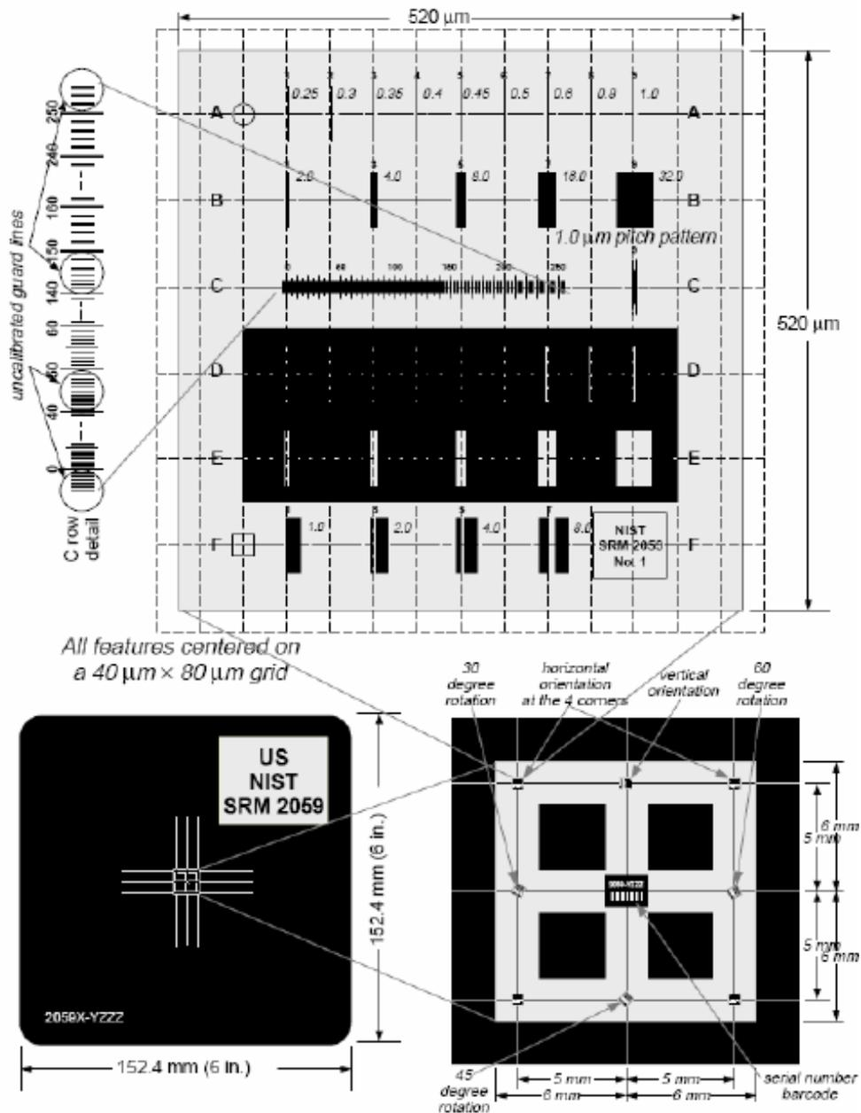
**Figure 1.** Schematic illustration of the layout of SRM 2059 – the current NIST binary photomask standard. The isolated line features are in rows A and B, and the isolated space features are in rows D and E. Both feature types range in width from 0.25 μm (the A1 and D1 features) up to 32 μm (the B9 and E9 features). (Note that due to AFM scale uncertainty, only features up to 8 μm width were measured in this work.)
