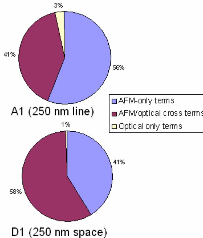
**Figure 3.** Origin of relative contributions to final combined variance for the 0.25  $\mu\text{m}$  line and space targets which are A1 and D1, respectively. The combined expanded uncertainty in the linewidth of both features is approximately 14 nm ( $k = 2$ ). Note that the optical-only share (type A) is a small fraction, but correlation of the optical and AFM results contributes roughly on par with the AFM-only share – which was due to tip calibration.
