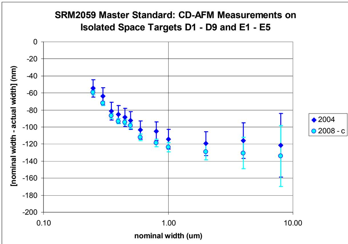
**Figure 5.** New and original CD-AFM reference measurement on the isolated space targets of SRM 2059 – ranging from 0.25  $\mu\text{m}$  width (D1 feature) up to 8  $\mu\text{m}$  (E5 feature). The error bars represent expanded ( $k = 2$ ) uncertainties, which have been reduced by approximately x4 for the smallest features.
