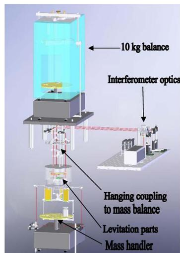
Fig. 6. Main components of the next-generation magnetic levitation mass comparison system.
