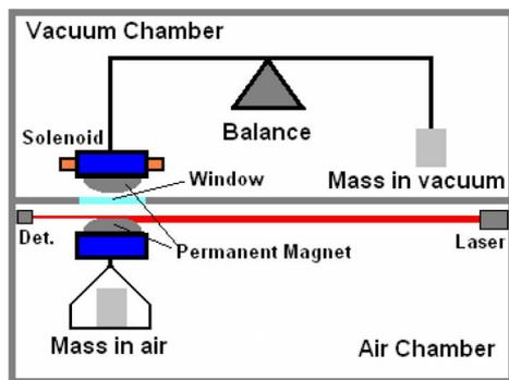
Fig. 1. Schematic of a magnetically coupled mass comparison system that functions in air and in a vacuum.
