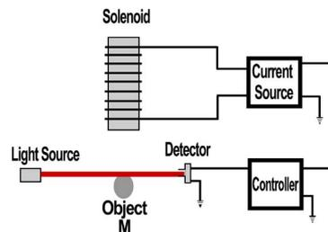
Fig. 2. Simple magnetic levitation system. A shadow detector and a feedback controller are used to suspend a ferromagnetic ball.
