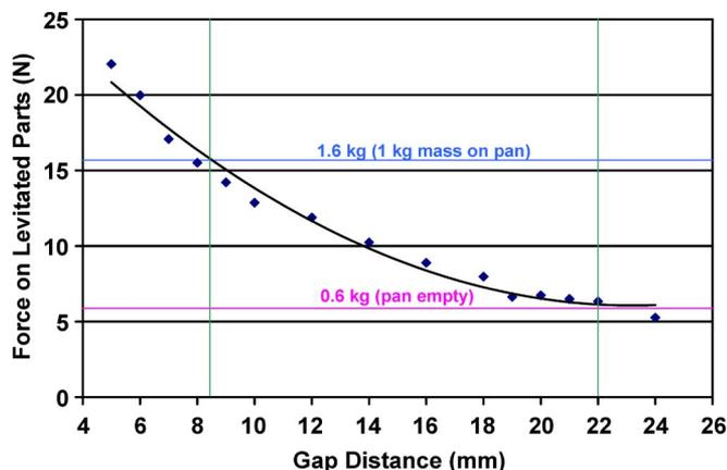
Fig. 5. Magnetic force as a function of distance between the fixed pole and the pole attached to levitated parts (gap distance).
