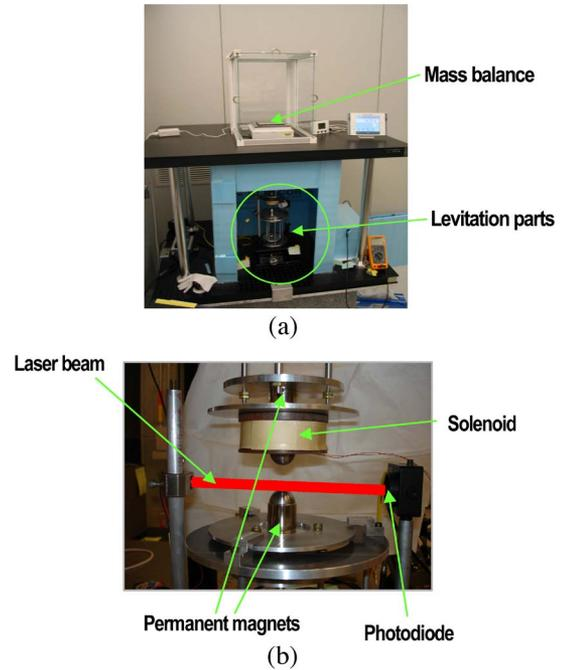
Fig. 4. (a) Proof-of-concept apparatus for a levitation mass comparison system. (b) Close-up of levitation parts in a proof-of-concept apparatus.
