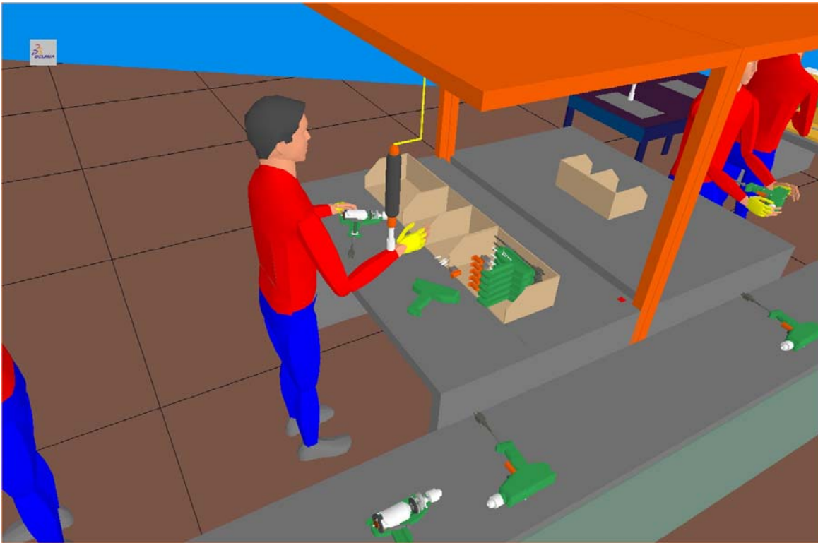
Figure 1. Simulation of the assembly of handheld power tools
