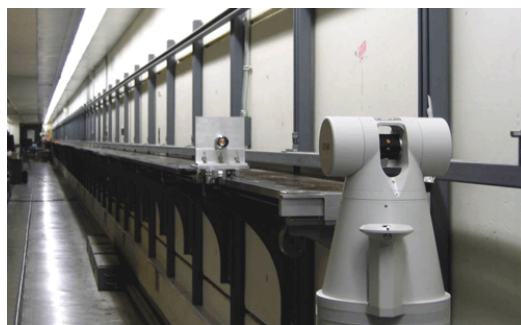
Figure 1. The NIST 60 m laser rail facility viewed from the tracker under test end; note the movable carriage with retroreflector.
