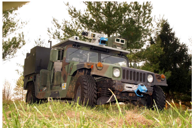
Figure 2. The roof-mounted laser rangefinder. The bumper-mounted rangefinder was not used in the results reported in this paper.
