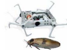
Fig. 5. Mini-Whegs and its relative size as compared to a cockroach
