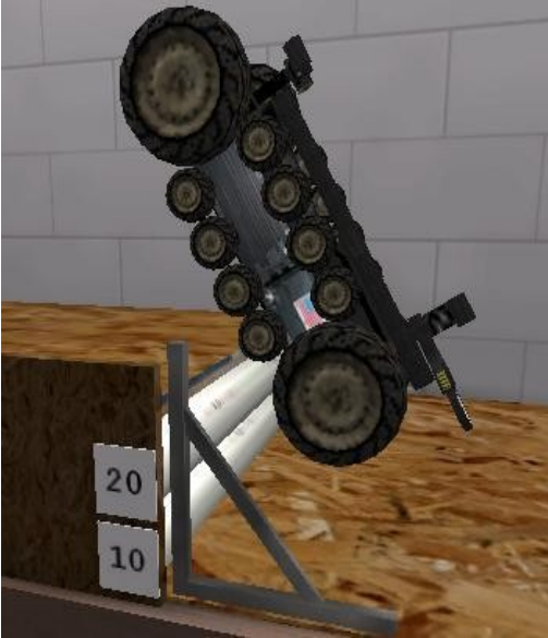
Fig. 11. Talon Model Climbing of Pipe in Reverse
