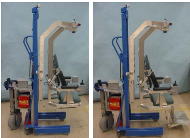
Figure 2 – Photographs of the HLPR Chair in patient access (left) and mobility (right) configurations. The left photo shows the footrest retracted to easy chair access and the right photo shows the footrest deployed for mobility.
