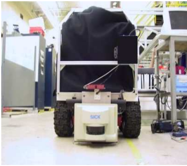
Fig. 5. Experimental setup of the AGV, the scanning laser rangefinder, and the range camera.
