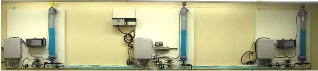
Figure 4 - Water Distribution SCADA System
