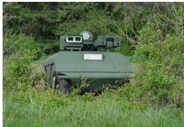
Figure 1: The Demo III XUV is a hydrostatic diesel, 4 wheel drive, 4 wheel steer vehicle capable of autonomous navigation in unstructured and off-road driving conditions. The LADAR is shown in white.
