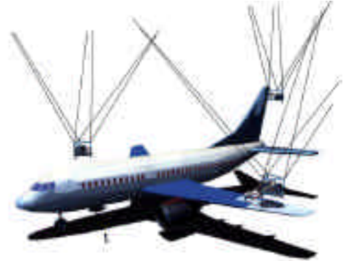
Figure 1. Cable robots capable of six-degree-of-freedom motion, in an aircraft maintenance application. Hoists on the moving platforms lengthen or shorten cables in a coordinated way to move the platform in an intuitive coordinate system. Computer control calculates the transformations from user coordinates to cable lengths.
