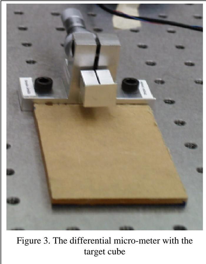
Figure 3. The differential micro-meter with the target cube
