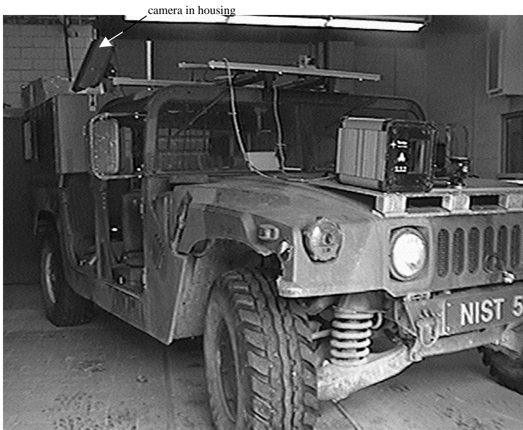
Figure 6. Picture of downward pointing camera mounted on side of vehicle.
