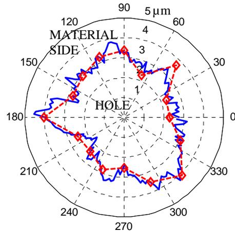
FIGURE 7 Radial form data from a knife-edge aperture used in NIST round robin comparison. 180 sampling points per trace, average of 10 traces shown in solid line. Additionally, the dashed-diamond line represents 16 sampling points measured with the probe on a CMM. 2D point coordinates were determined at each sampling location. The residuals from a Least Squares best fit circle are shown here.
