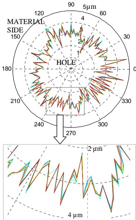
FIGURE 6 Radial form data from a knife-edge aperture. 180 sampling points per trace, 10 traces are shown. The repeatability at any location is only of the order of 62 nm. The out-of-roundness of this artifact is approximately 2  $\mu\text{m}$ .
