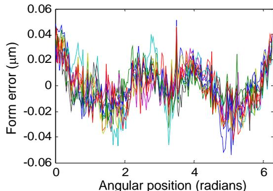
FIGURE 2 Radial form data from 3 mm sphere
