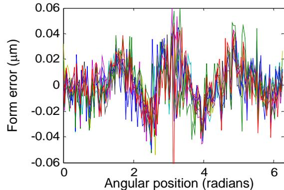
FIGURE 3 Radial form data from 3 mm sphere at the  $180^\circ$  position of a full Donaldson reversal, with 180 sampling points per trace and 10 traces
