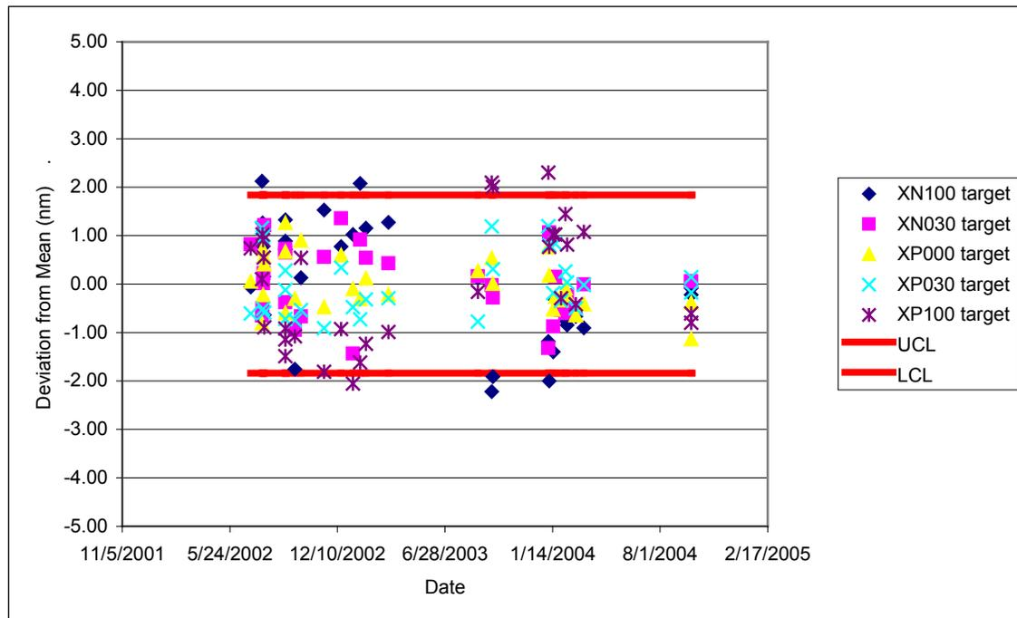
Figure 4 – FF control chart (UCL – Upper Control Limit, LCL – Lower Control Limit)
