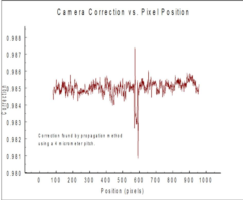
Figure 7 – Plot of CCD pixel pitch calibration factors versus position
