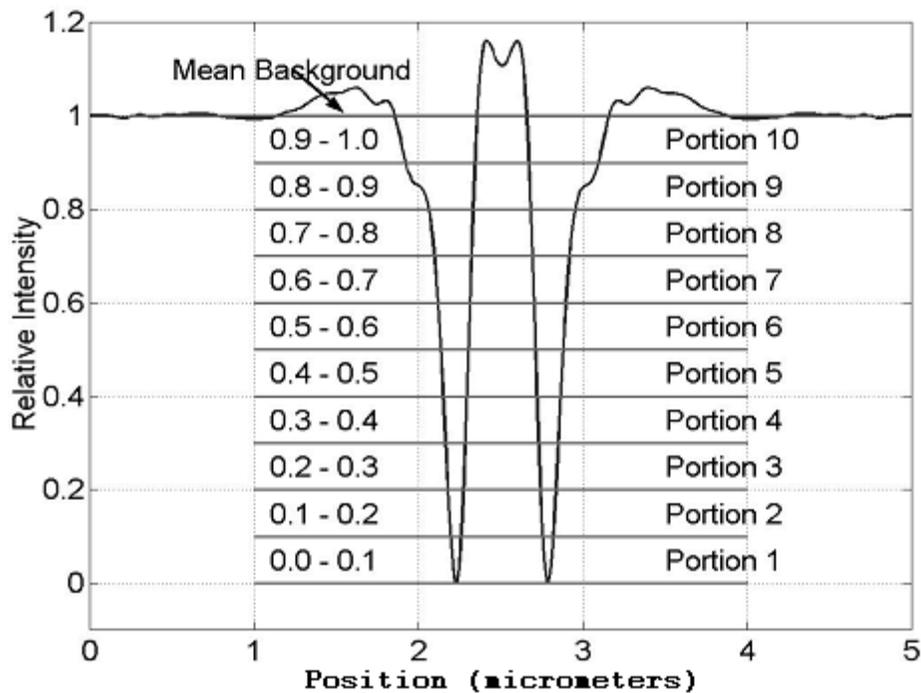
Figure 8 – Levels of Truncation on one leg of an OL target.
