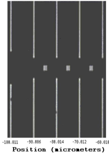
Figure 10 – Image at 100X of the SRM 2800 used to calibrate the camera/microscope scale.
