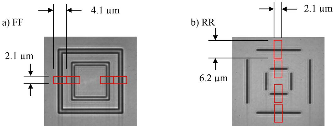
Figure 3 – Window dimensions for FF and RR targets
