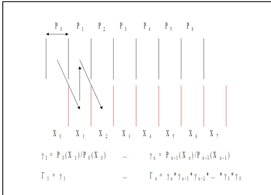
Figure 6 – Diagram of 1-d self-calibration algorithm
