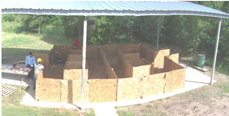
Fig. 6 Mobility/endurance test method layout
