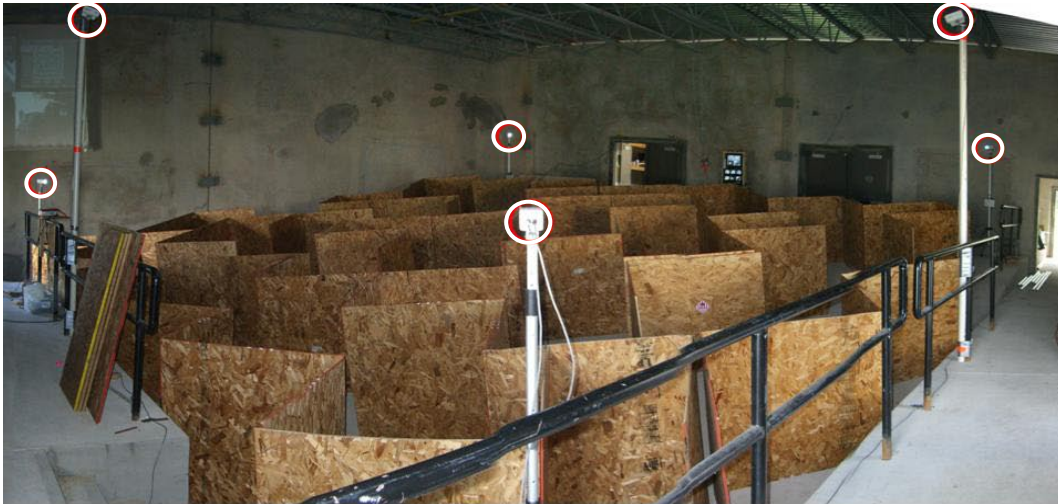
Fig. 3 UWB Tracking System Receiver Positions (circled in red) around the Maze Test Method
