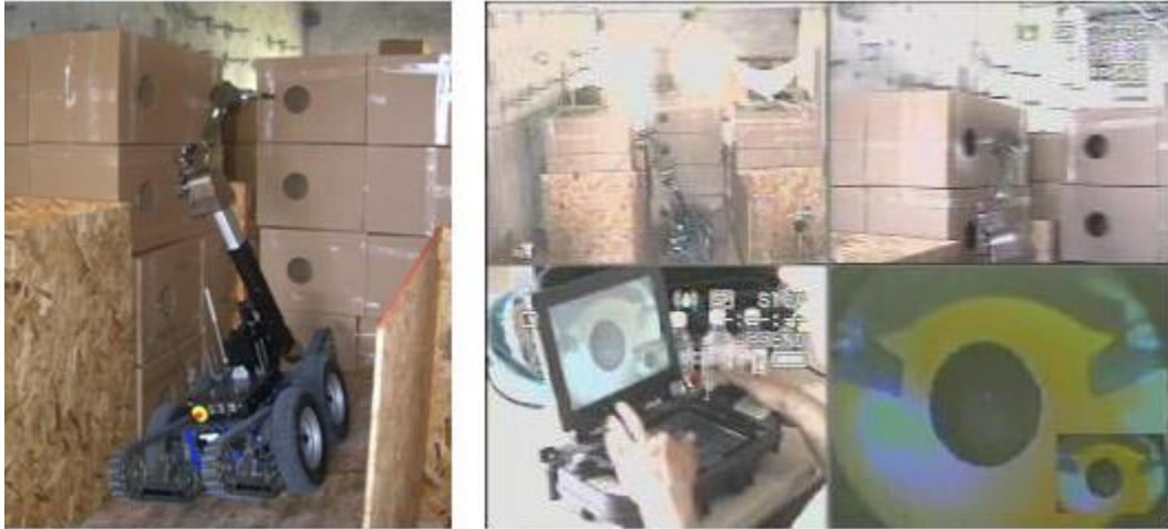
Fig. 5 a) Robot participating in the directed perception test method and b) resultant quad screen video
