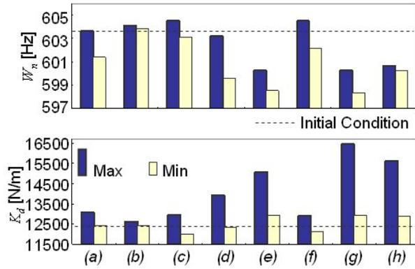
Fig 9: Maximum and minimum values of tool point dynamics according conditions in milling operations
