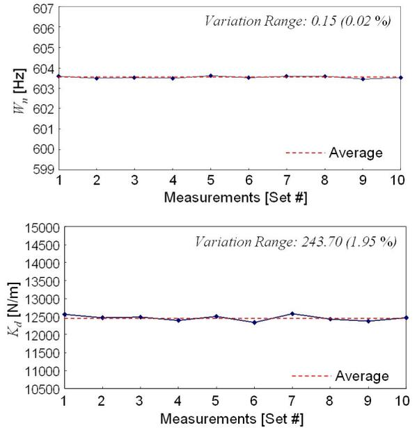
Fig 2: Tool point dynamics of initial condition
