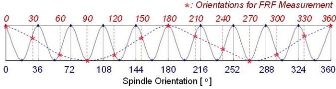
Fig 3: Expected variation in FRF measured at every 30° orientation of spindle with twenty-ball bearing
