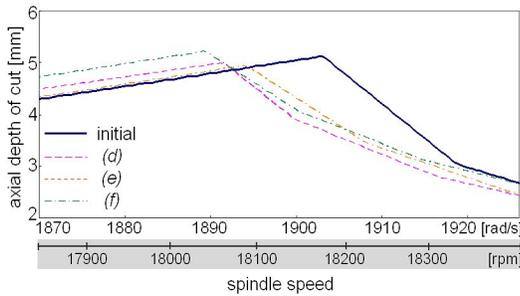
Fig 13: Changes of stability lobes with significant changes in best speed
