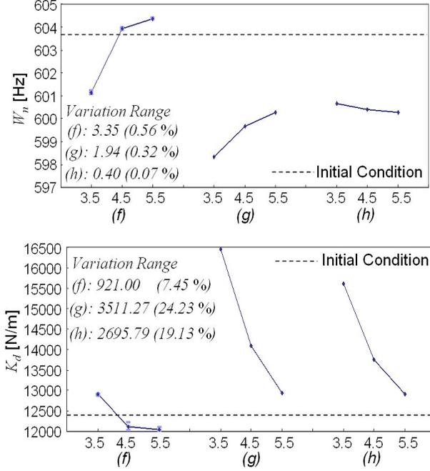
Fig 8: Changes in tool point dynamics by torque variations between tool and holder
