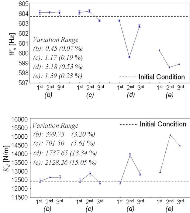
Fig 7: Changes in tool point dynamics by tool and tool assembly changes in spindle
