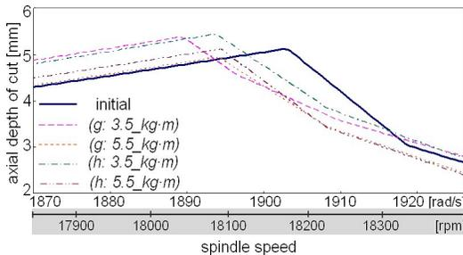
Fig 14: Changes of stability lobes with significant changes in best axial depth of cut
