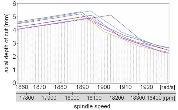
Fig 15: Stable region considering changes in machining stability
