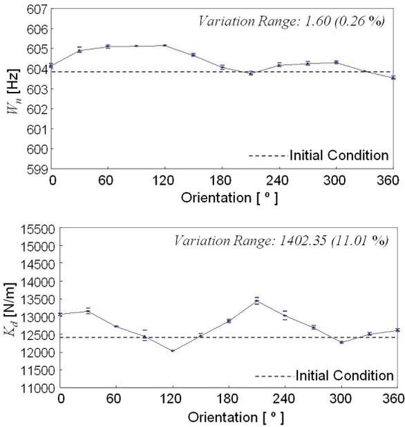
Fig 4: Variations in tool point dynamics according to spindle orientations
