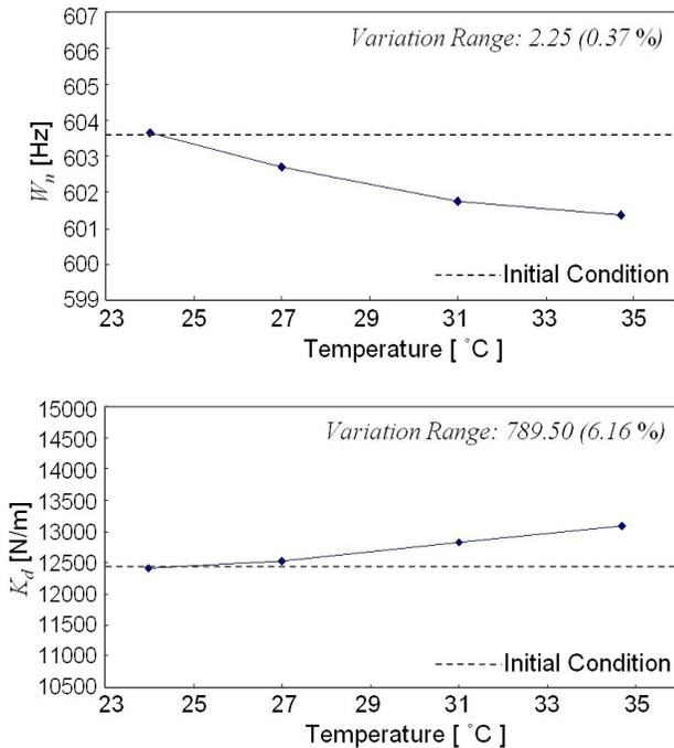
Fig 6: Changes in tool point dynamics in warmed up tool-holder-spindle system
