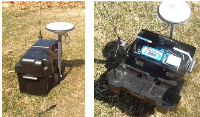
Figure 5. The ground truth data logging unit consists of a GPS receiver with memory card for logging data, a differential GPS data link radio, antennas, and battery power.
