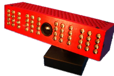
Figure 1 - The TOF 3D range image camera. The camera simultaneously generates intensity images and range information of targets in its field-of-view at a rate of 30 Hz with an active range of 7.5 m [25].
