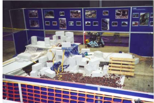
Figure 4a: Simulated rubble pile and unstable flooring in the NIST Red arena
