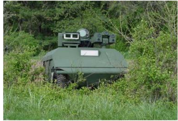
Fig. 1. The Demo III eXperimental Unmanned Vehicle can drive autonomously at speeds of up to 60 km/h on-road, 35 km/h off-road in daylight, and 15 km/h off-road at night or under inclement weather conditions. The Camera is mounted above the LADAR shown in white.
