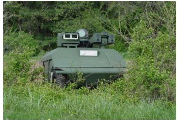
Fig. 4. The Demo III eXperimental Unmanned Vehicle can drive autonomously at speeds of up to 60 km/h on-road, 35 km/h off-road in daylight, and 15 km/h off-road at night or under inclement weather conditions.
