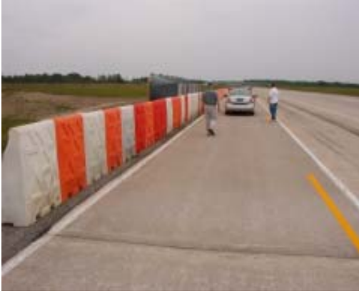
Figure 8. Test set-up for road departure toward jersey barrier.
