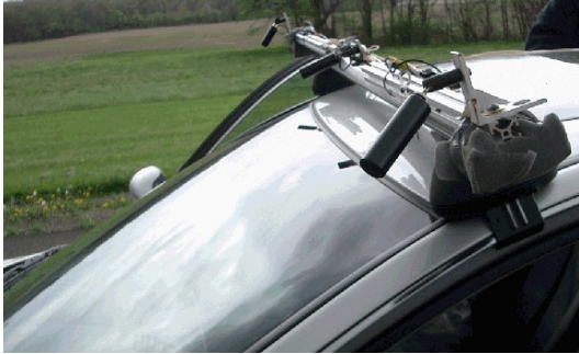
Figure 1. Three weatherproof cameras mounted on roof rack.
