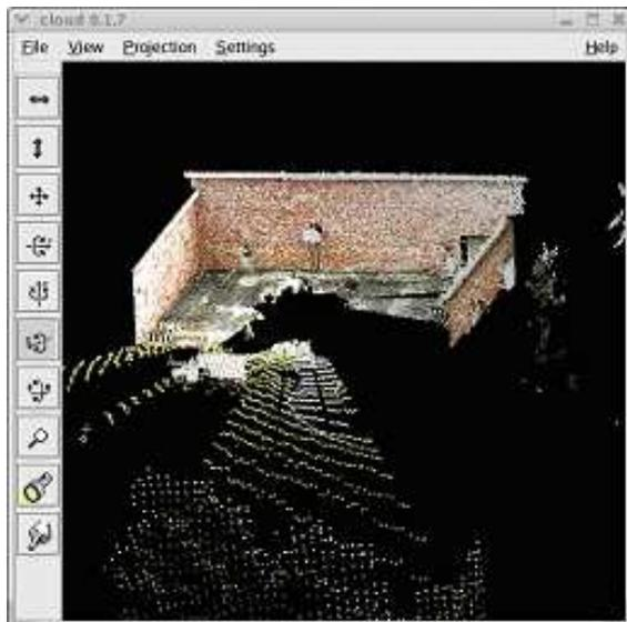
**Figure 2** Data from a scan of orthogonal walls using the Riegl lidar.
