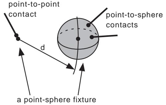
Figure 8. CONTACTS TO A POINT-SPHERE FIXTURE
