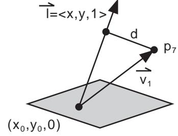
Figure 5. SHORTEST DISTANCE BETWEEN A POINT AND A LINE
