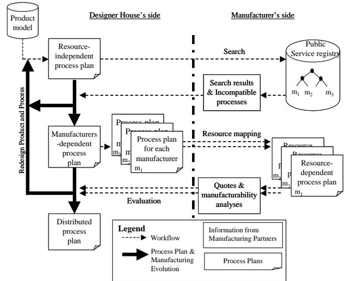
Fig. 2 Process information workflow for collaborative planning and manufacturing
