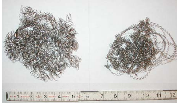
Fig. 7: The \text{AlMgB}_{14} tool insert (on the right) produces a much more tightly curled chip (scale in inches)
