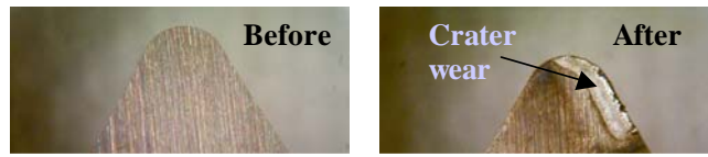
a) Tool wear for WC-Co insert's material, test J-1
